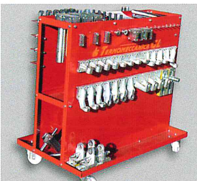
Carrello porta dima / Subsidiary JIG trolley
